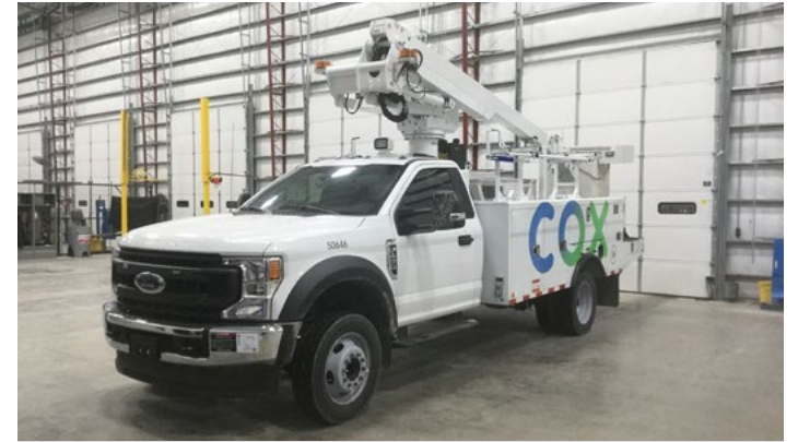
Our ALTEC JEMS 2A bucket trucks are electric, use their battery system to monitor cab climate and only start the truck when required.
